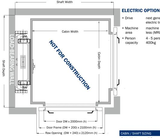
CABIN / SHAFT SIZING Cabin Width + 360 = SW Cabin Depth + 160 = SD
